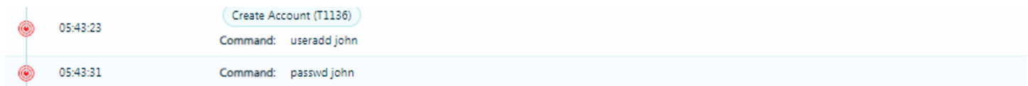
Fig. 3.3 Threatwise alert details of hackers newly creating users and setting passwords on Linux sensors.
